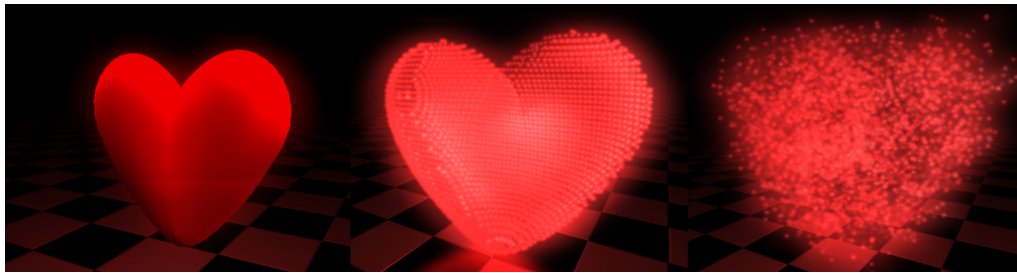
Figure 7: Screenshots of our FX demo HeartBreaker . From left to right: Solid model (5000 triangles); Point cloud representation (1872 points, in a 256 \times 64 \times 64 grid, first iteration: 90 ms, subsequently: 25 ms); Particle explosion effect.
