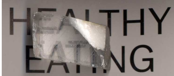
Figure A.1: A birefringence crystal (calcite) showing the double refraction of the light.
