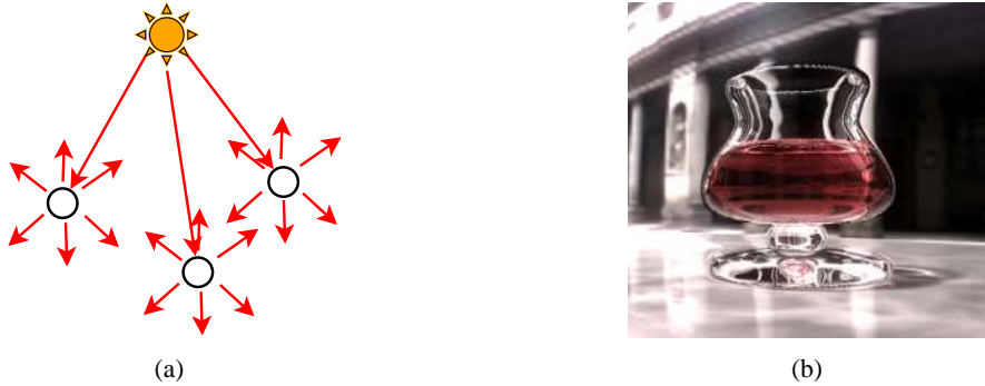
Figure 3.3: (a) Scattering occurs when light originating at the light source scatters on material impurities, e.g. dust particles. (b) Wine glass showing refraction and attenuation. Wine attenuates green and blue components of the light resulting in a red colored fluid.
