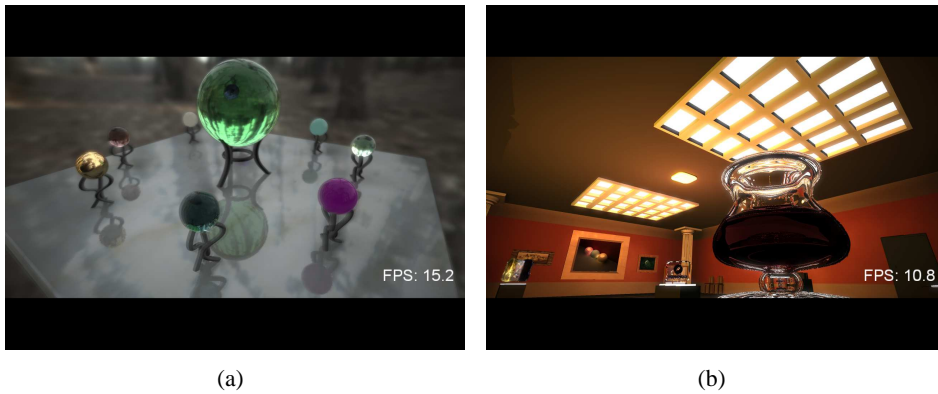
Figure 7.5: (a) Scene showing up to 9 objects simultaneously. The big sphere in the middle has a resolution of 128^3 voxels, while the small spheres surrounding it are composed of only 32^3 voxels. The rendering speed in this scene varies between 9 FPS (when the big sphere fills out the complete viewport) and 60 FPS (whenever only the small spheres are visible). Frame rate of the screenshot is 15.2 FPS. (b) A screenshot from the museum scene, showing all refractive objects simultaneously. The objects exhibit various optical effects. Their resolution is 128^3 voxels, with up to 6 volume data textures for each object. The rendering speed is 10.8 FPS.
